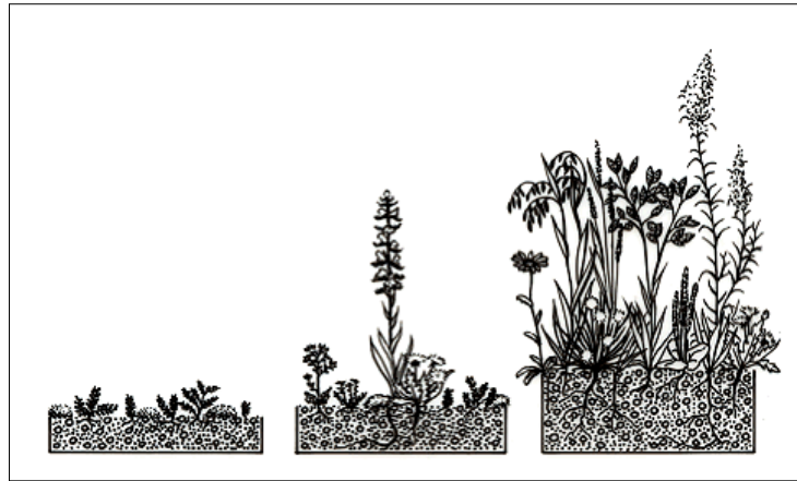
Illustration showing the diversity of plants supported with substrate depths of 6, 12 and 20cm (taken from Brenneisen, 2006 18 )
